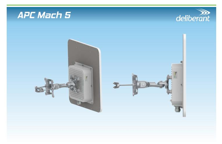
The APC Mach 5 presents a 5 GHz point-to-point product with superior performance building long distance links. This product is equipped with an extreme output power (up to 29 dBm) 802.11n radio that was created with a unique hardware design and coupled with a reliable, feature-rich operating system. This device also has a robust, IP-67 compliant enclosure which is combined with a high-gain dual-polarized panel antenna. The APC Mach 5 is generally designed for PTP applications, but can
